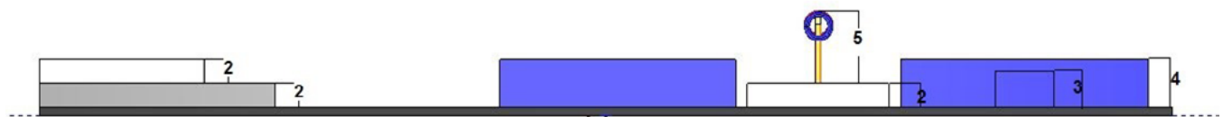
Figure 5: Back view of challenge board with dimensions. All measurements are in inches. The red and blue rings are both 2 inches in diameter and \frac{1}{4} inch thick.
